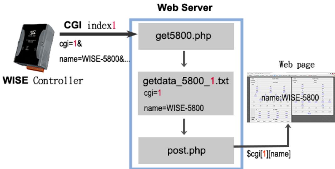
When the WISE controller receive a CGI command, it will retrieve the data specified in the command, by using get5800.php and get7126.php, the data will be transferred into txt file and will be saved in the form of getdata\_5800\_1.txt (indicating this txt file includes the data retrieved from WISE-5800 that is required by CGI command 1)
